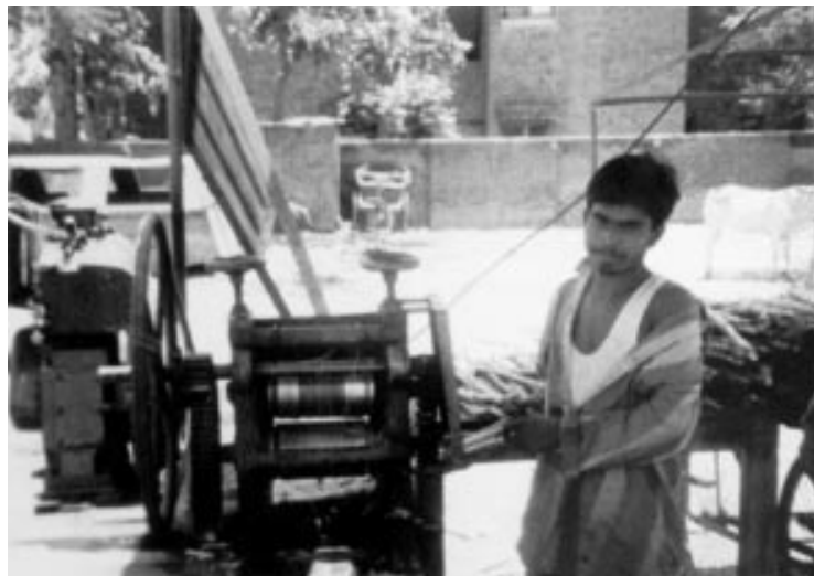
Figure 1 Sugarcane crusher with single operator showing no safety features.
