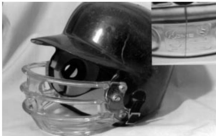
Figure 1 A baseball face guard consisting of a polycarbonate arch affixed to the ear flaps of a standard batter's helmet. Inset: close up photograph of a fracture in the arch caused by a pitched ball impact while worn by an 8 year old face guard team batter. This product was manufactured to the specifications of ASTM F910, which prevents facial contact from a baseball fired at 69 miles per hour.<sup>10 11</sup>
