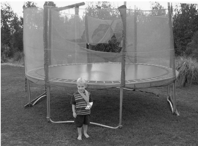
**Figure 1** A typical consumer trampoline and enclosure after less than 3 years of use. The pads have deteriorated and been removed, the enclosure net is torn. The subject bounced through the hole in the net and fell to the ground, fracturing his wrist (with permission from Dr S Gooch, University of Canterbury, New Zealand).
