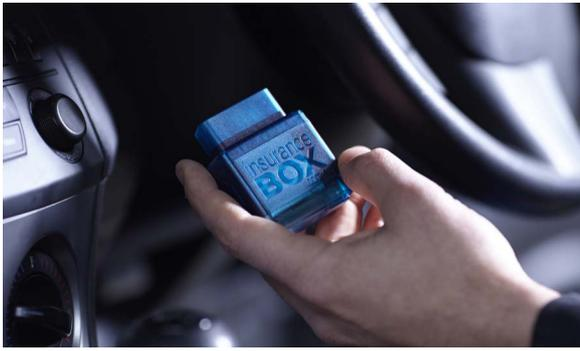
**Figure 1** Telematics device.
