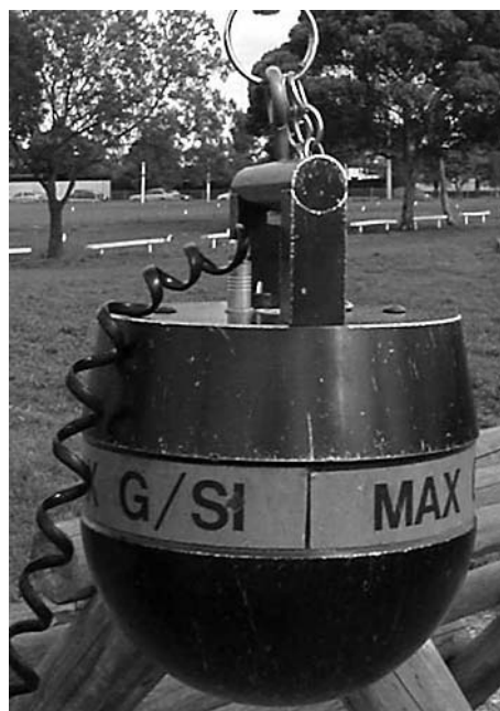
Figure 2 The drop test headform used for peak deceleration and HIC measurements.
